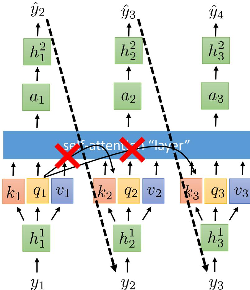
**At test time** (when decoding), the **inputs** at steps 2 & 3 will be based on the output at step 1...
